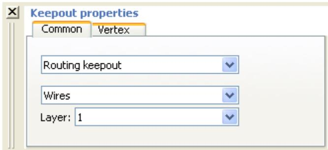
Next, set the keepout role: **Routing Keepout** or **Placement Keepout**.
