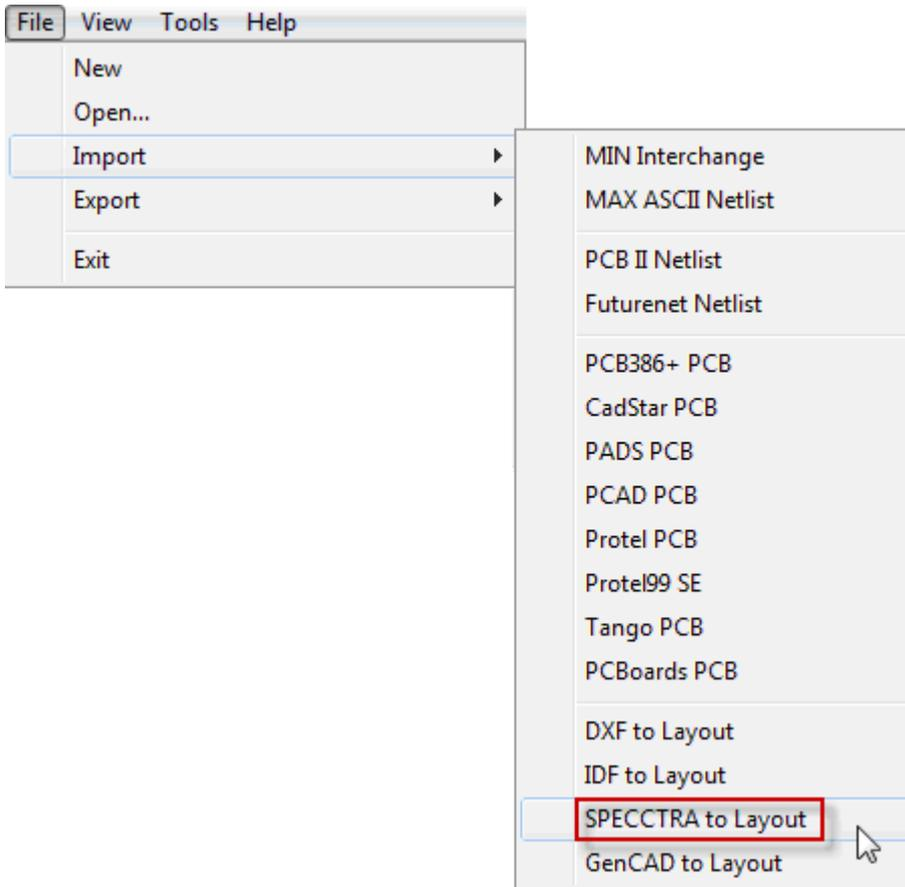
In the **SPECCTRA to Layout** dialog box that opens, specify the input and output files correctly:
