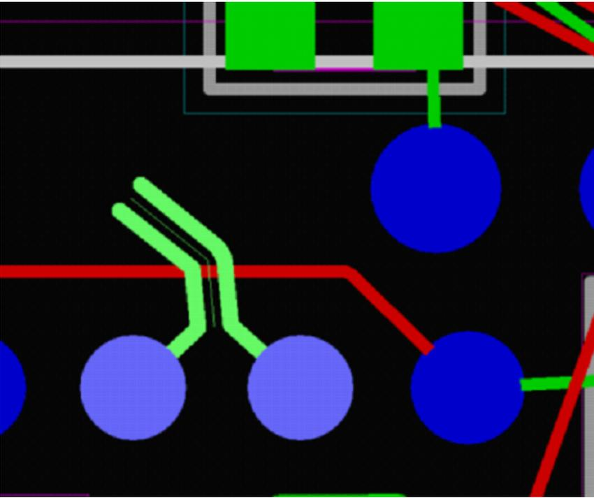
If the selected segment belongs to an unzipped wire, then pressing the **X** key selects the segment up to the slider. Pressing **X** again selects the entire wire, as shown in the following screenshots:
