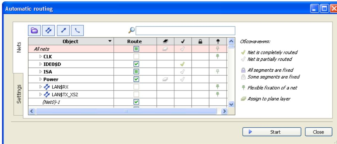
Before routing is first started, the autorouting control panel has two tabs: [Nets](#) and [Settings](#). After routing has been started at least once, the [Variants](#) tab is added.
