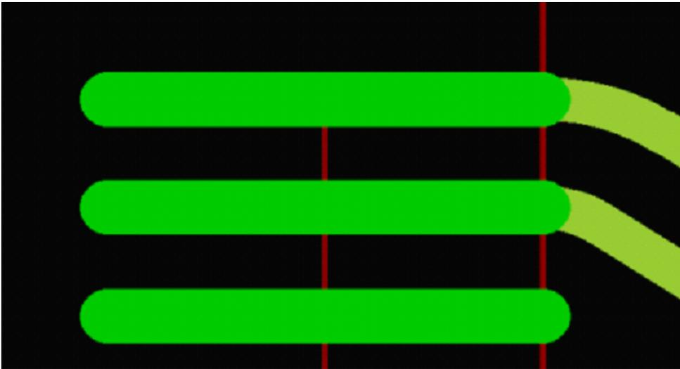
During wire switching, if the pads are planar and located on different layers, the wires remain unconnected (similar to changing the placement side of a planar component). If the second click does not hit a pad in the selected group, the first pad is deselected, and the command is not performed.
