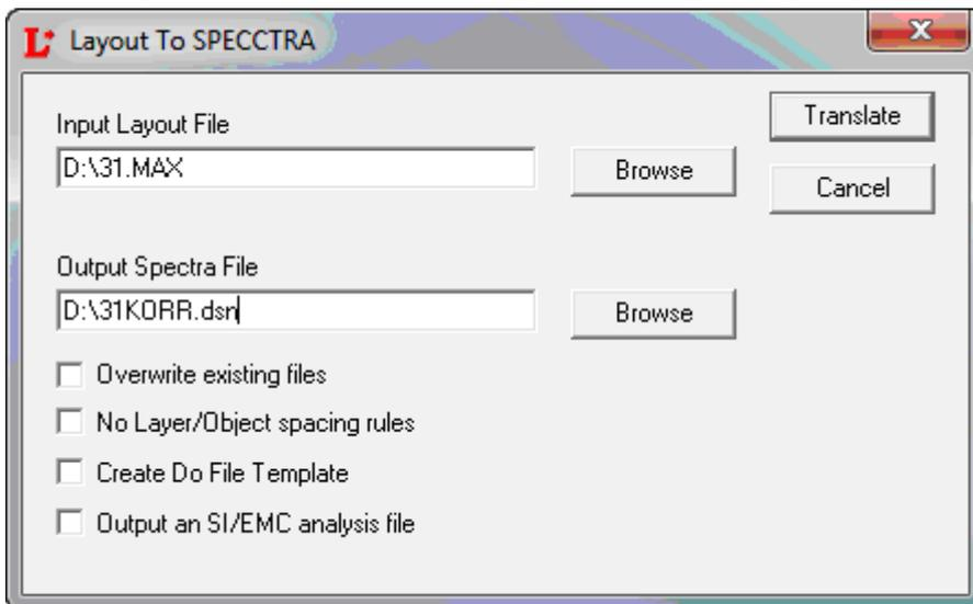
Use the **Browse** button next to the **Input Layout File** box to specify the **\*.max** project file. In the **Output Spectra File** box, change the extension from **.cct** to **.dsn**. Then click **Translate**.
