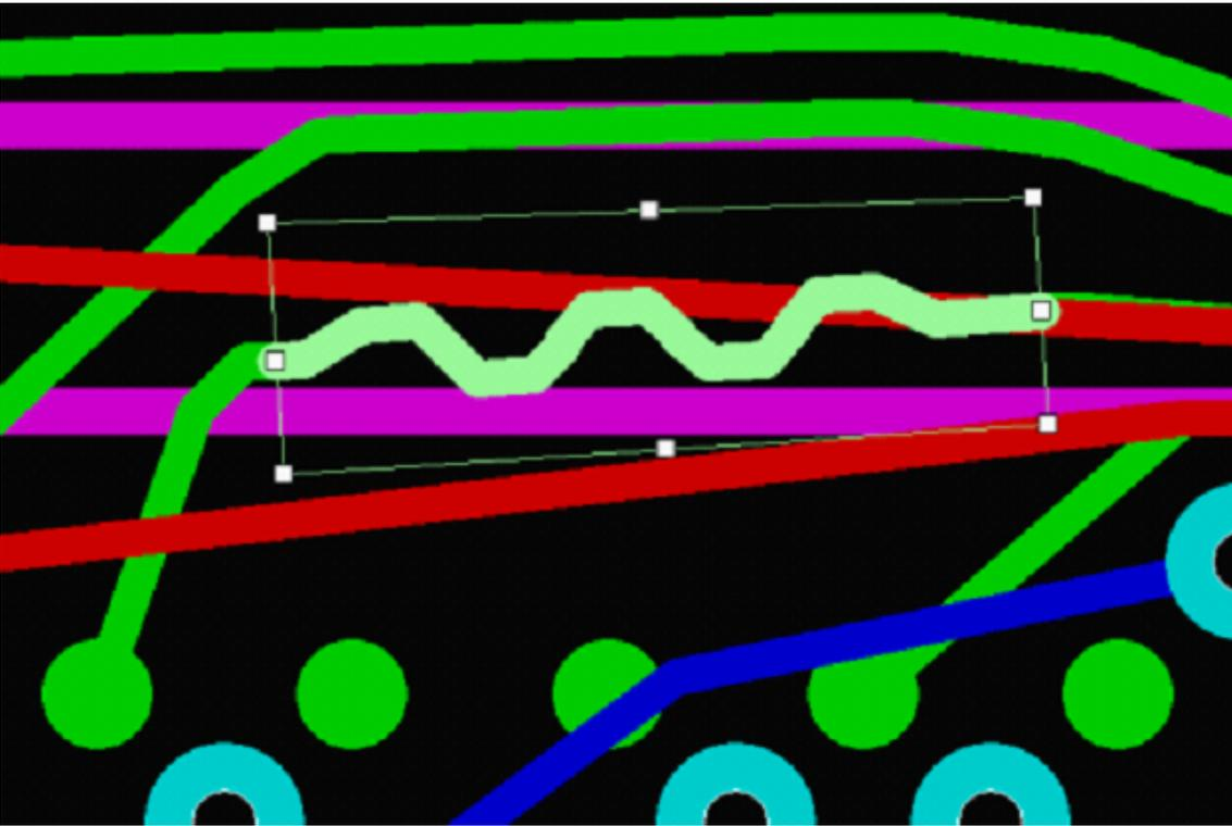
By moving the markers at the base vertices, you set the base length and the angle of the adjacent lateral side.
