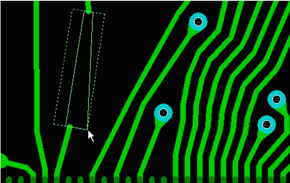
After an area stops being narrow, subsequent marker moves give it a trapezium shape.
