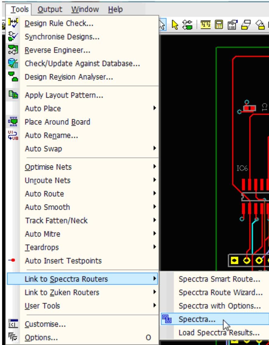
In the dialog box that opens, specify where to save the **.dsn** file. Make sure the **Launch Router** option is turned off.
