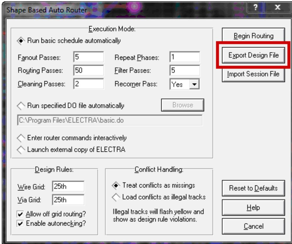
Save the file as **.edf**. To import a **.edf** file into **TopoR**, use the Spectra file type.
