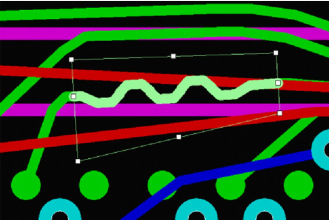
By moving a marker in the middle of a lateral side, you move the side along the bases.
