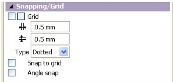
When snapping is enabled, the segment incident to the vertex you are moving rotates in 45-degree steps. To enable and disable snapping, press the **O** key. When you move a vertex shared by two segments, only one of the segments uses snapping. To select which of the segments snaps, press the **P** key.
