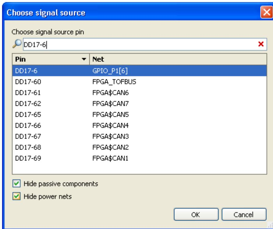
The search string can contain multiple substrings separated by spaces. The search works on the names of components, pins and nets.
