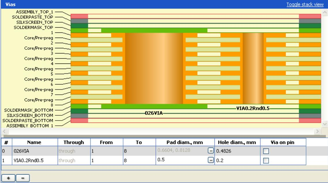
The screenshot shows the Vias dialog box with a stack view and a table of via parameters. The stack view shows layers from ASSEMBLY\_TOP\_1 to ASSEMBLY\_BOTTOM\_1, with two vias labeled 026VIA and VIA0.2Rnd0.5. The table below shows the parameters for these vias.
