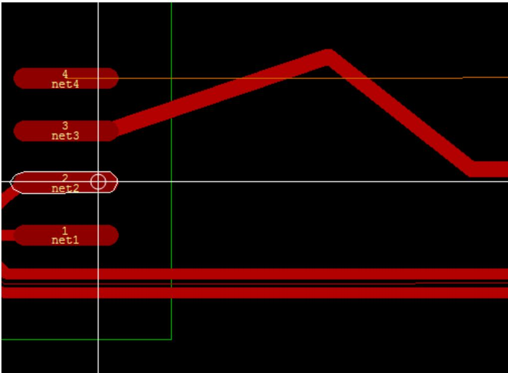
Clicking at this time selects the first object and marks the current cursor position as point A. After that, the tool is ready for selecting the second object. Until you select it, the ruler draws a line from point A to the current cursor position. After the second object is selected, the tool calculates the distance and draws a corresponding line.
