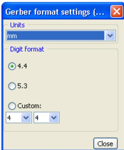
This dialog box lets you configure some parameters of Gerber output. Set the units to use (mm or mil), and specify the format for numbers (such as “4.4”, meaning four integer digits and four decimal places, or “5.3”, or a custom format).
