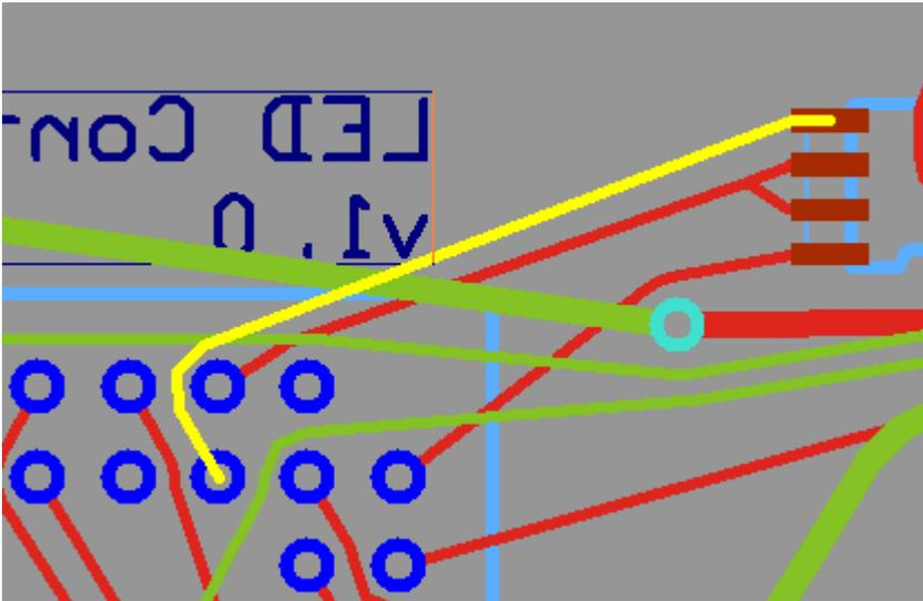
The message bar contains warnings about non-fixed elements that are over the edge of the board. At the same time, clearance violations are highlighted. The listed elements should be either fixed or moved to eliminate violations. This makes the warnings and highlighting disappear.
