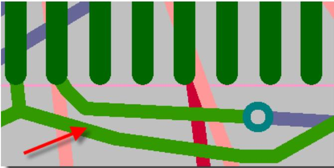
The “miscalculated” wire is marked with an arrow
