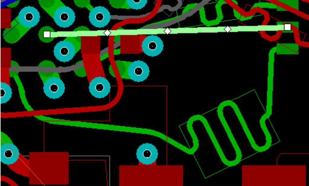
After wire straightening, confirm that the topological route of the modified fragment is correct and there are no topology violations: the route must not cross (in a topological sense) other wires on the same layer or pads belonging to other nets.
