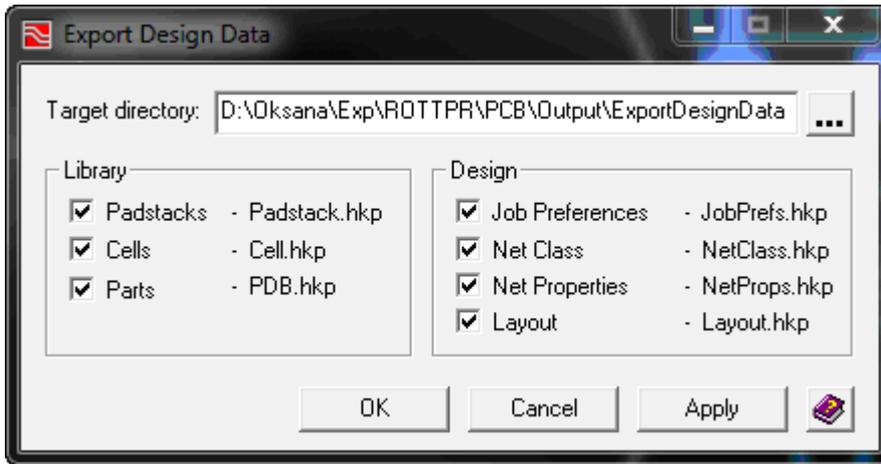
In older versions of Expedition (2007.2), **.hkp** files were written in plain text format and could therefore be easily imported into **TopoR**. In newer versions (2007.8) they are written in compressed binary format and need to be decoded before import. A converter utility for this purpose is shipped with Expedition. In a default installation, the path to the converter is as follows:
