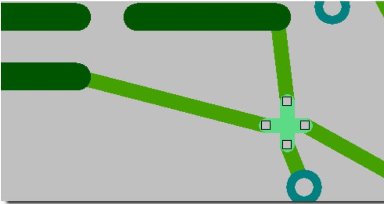
Nets are connected by fixing crossed elements
