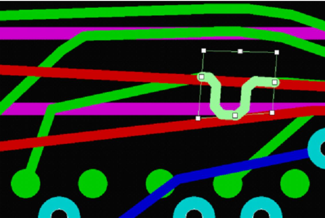
If the direction is not perpendicular, the trapezium is also rotated about the middle marker of the opposite base.
