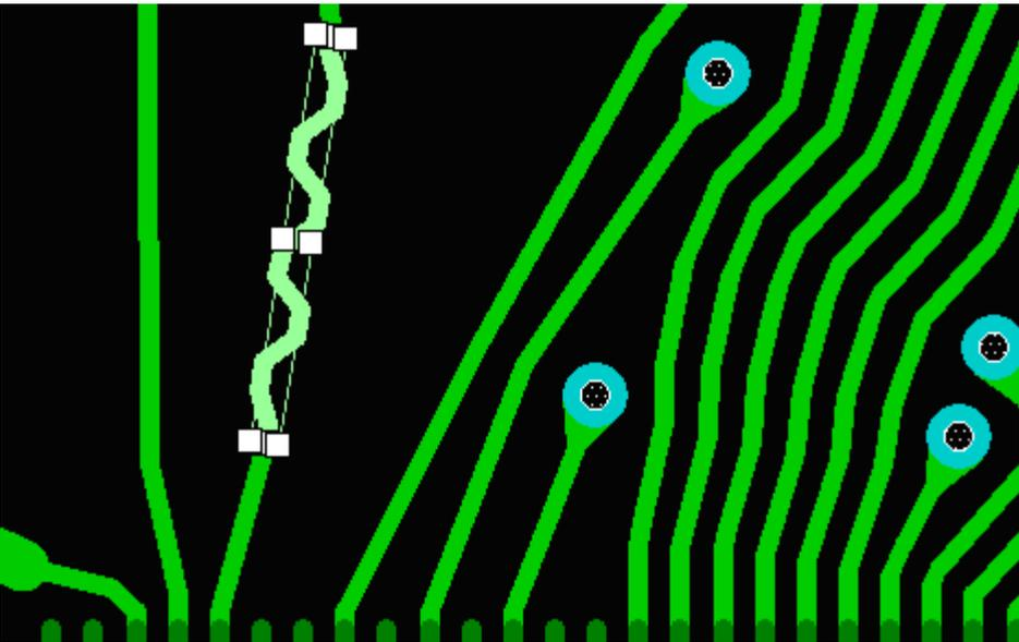
During a marker move, two areas are shown. The area indicated by a dotted line changes symmetrically.
