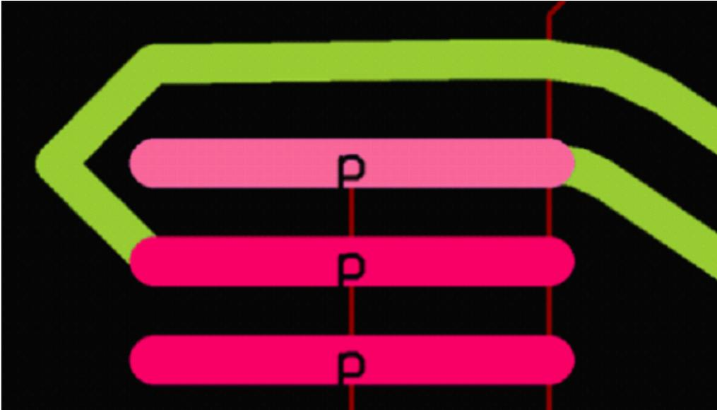
Clicking a pad in a group a second time reassigns pads. Net numbers are swapped for pads, and connected wires are switched.
