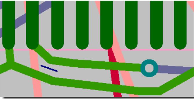
**Corrected: a routing keepout has been added**
