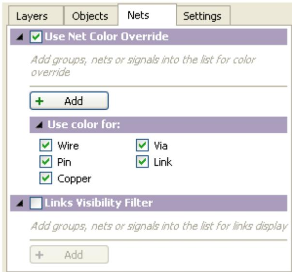
The **Nets** tab controls net display modes. The **Use Net Color Override** option helps group signals, nets or net groups by setting a custom color for them. If this option is enabled, you can select the objects to assign the custom color to wire, pin, copper, via or link.
