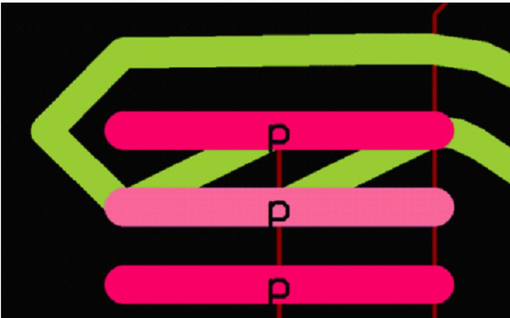
Normally, you need to edit wires to eliminate intersections with pads after this.
