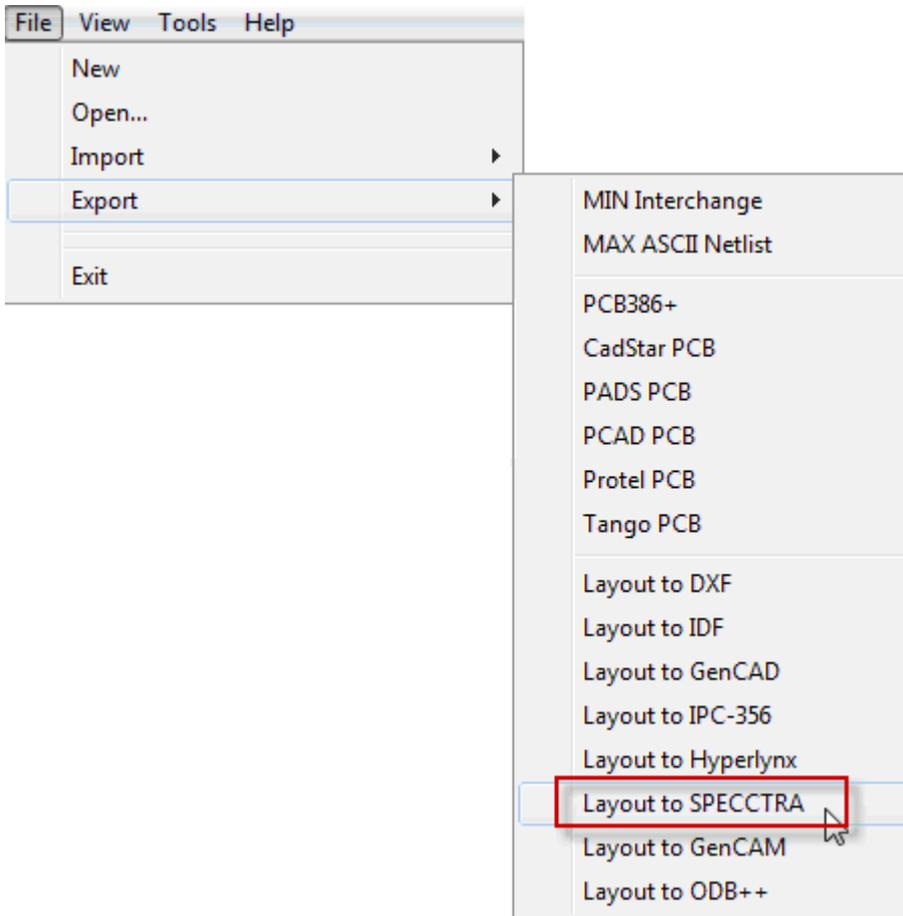
In the **Layout to SPECCTRA** dialog box that opens, specify the input and output files correctly:
