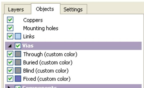
To edit a fixed object (for example, reshape a wire or shift a via), first unfix it. The fixed state of wires and vias is taken into account in all modes except Placement mode.
