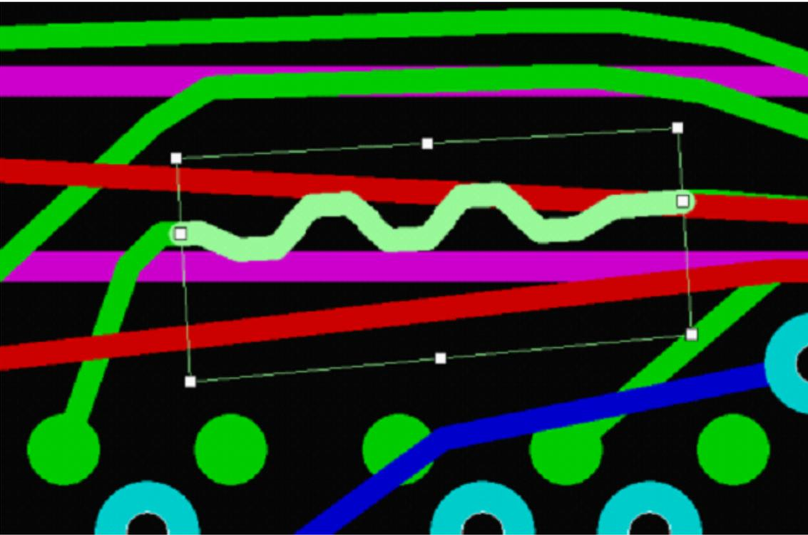
By moving a marker in the middle of a base perpendicularly towards or away from the opposite base, you make the lateral sides shorter or longer.
