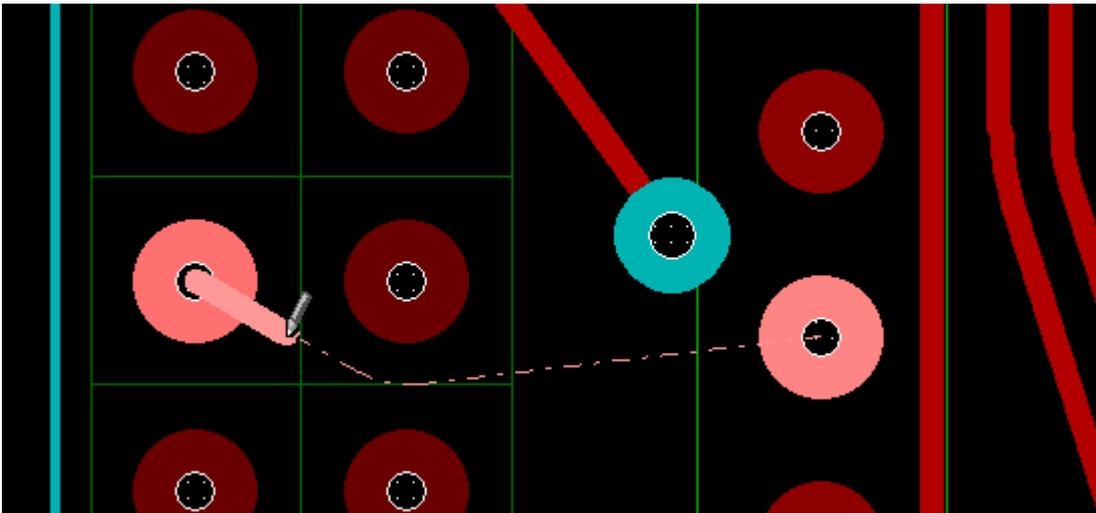
You can accept the discovered path (default shortcut: **Shift+Q**) to route the wire automatically. Otherwise, automatic searching will be performed for each new point under the cursor. The target can be changed by pressing the **Q** key if the path to the new target is shorter.
