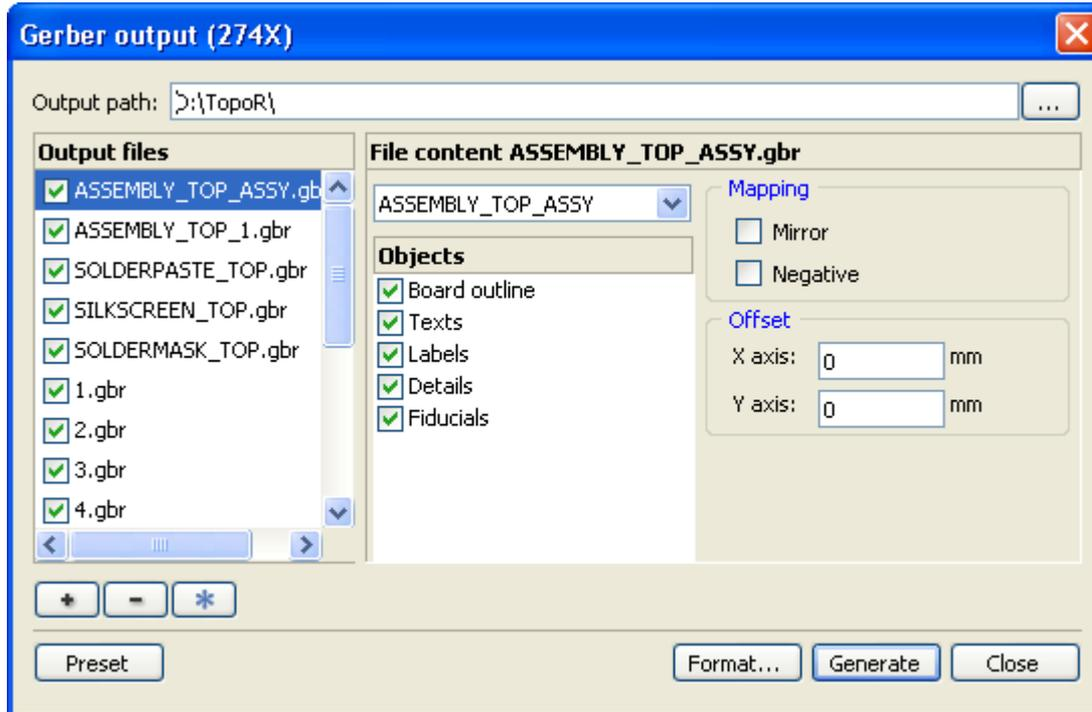
This dialog box displays two lists. The left list contains the names of files to be exported. The right list contains the layers to be included in the files.
