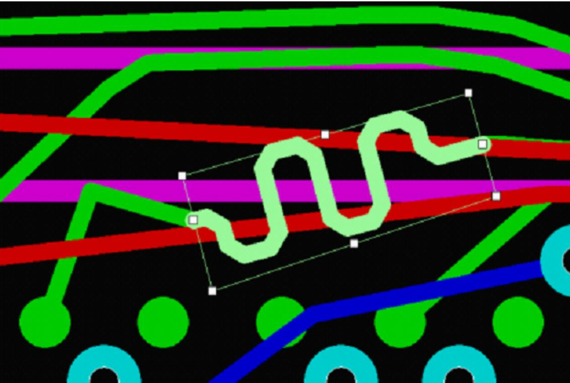
When you equalize wire lengths manually, the length and spacing of the inscribed serpent are taken from the **Delay** tab.
