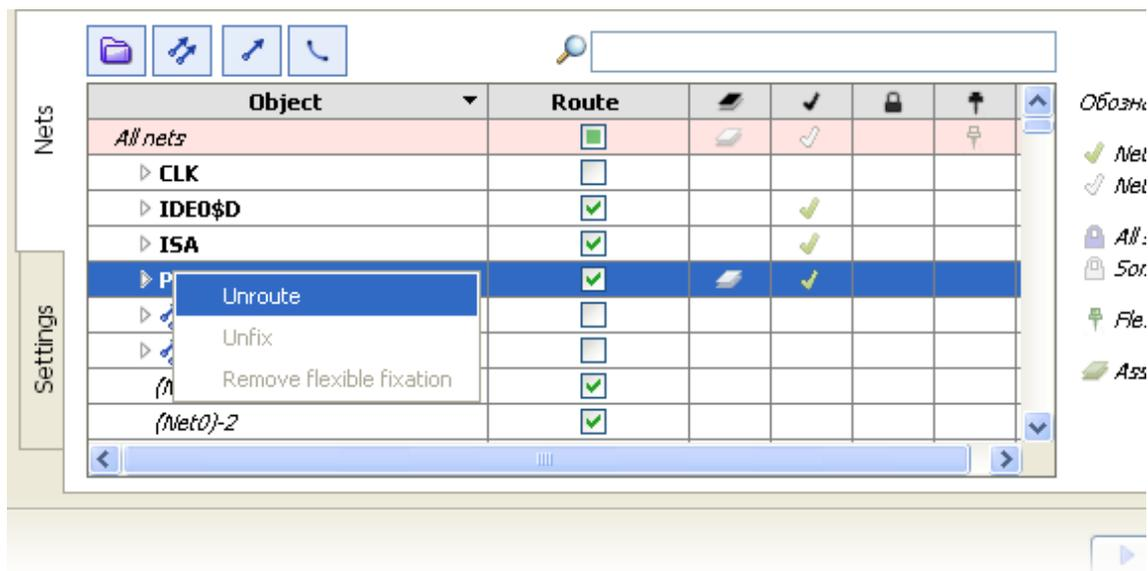
For example, all nets in the **ISA** net group are flexibly fixed, so the routing option has been disabled for it. Right-clicking the group lets you delete its layout, unfix it or enable routing for it.
