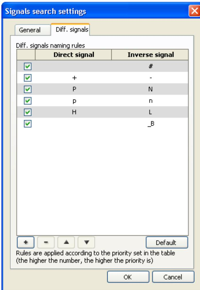
A DS net naming rule contains two substrings, one of which can be empty. Two nets match a rule if substrings represent the only differences in their names and both substrings are similarly positioned.
