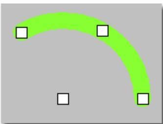
When the center marker of an arc is moved, the starting point and end point remain locked, the location of the center (and thus the arc radius) changes, the arc curvature does not change. When the middle marker of an arc is moved, the starting point and end point also remain locked, the location of the center changes, and you can change the arc curvature.
