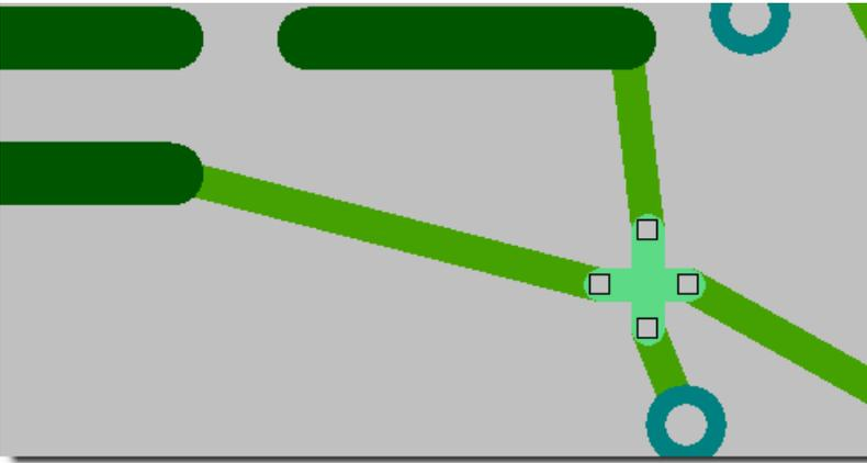
Nets are connected by fixing crossed elements
