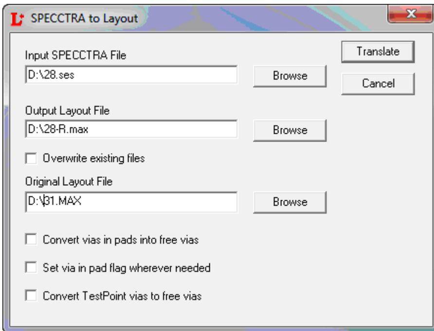
Use the **Browse** button next to the **Input SPECCTRA File** box to specify the **.ses** file. In the **Output Layout File** box, verify the name of the resulting **.max** file. In the **Original Layout File** box, specify the original **.max** file. Then click **Translate**.
