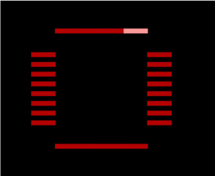
In this case, change the pad type in the component or in the library asset. That is, set different pad types for the different orientations.
