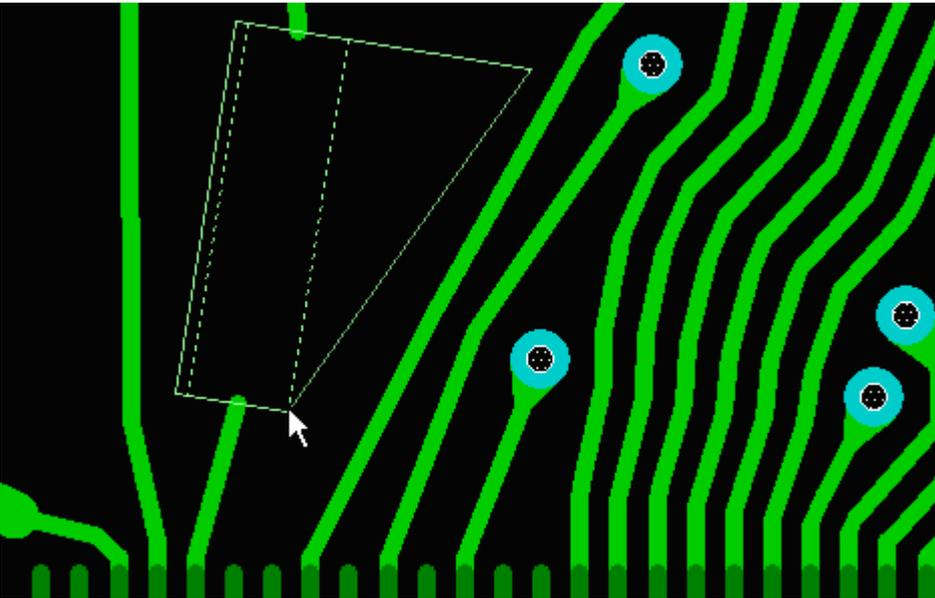
The minimum area width is 1.5 times the width of the wire.
