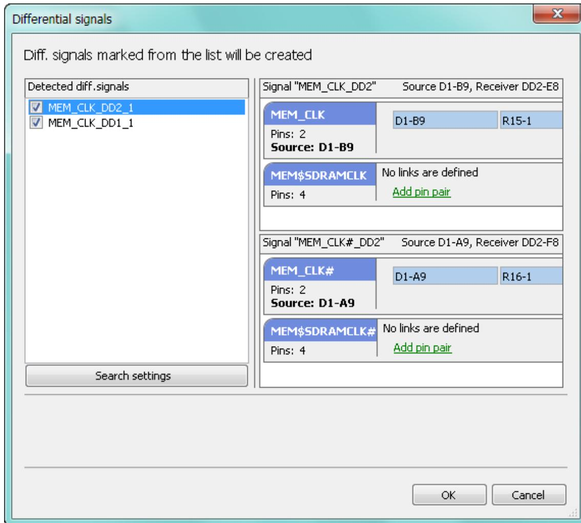
When you have selected the differential signals you want to create, information about the number of DSs to be created is shown at the bottom of the dialog box. When you click the **Create** button, the differential signals will be created.
