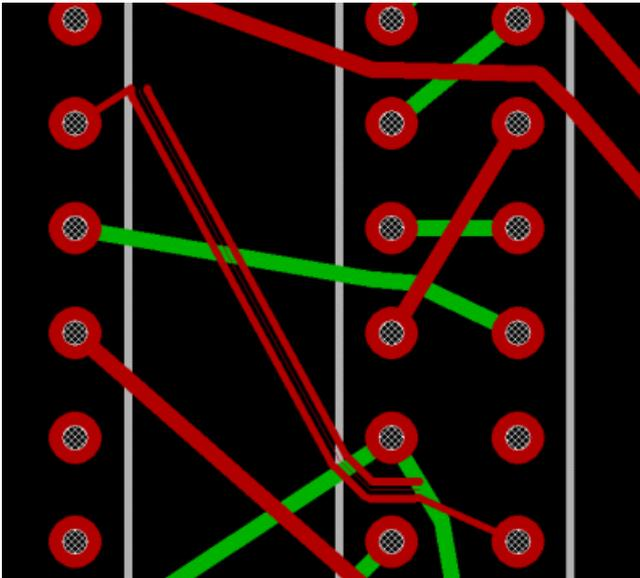
To switch layers, press the **L** key and select the next layer. As a result, a slider is automatically added on the current layer, and a pair of vias is added on the new layer, as well as wire segments connecting the vias and the corresponding slider pads.
