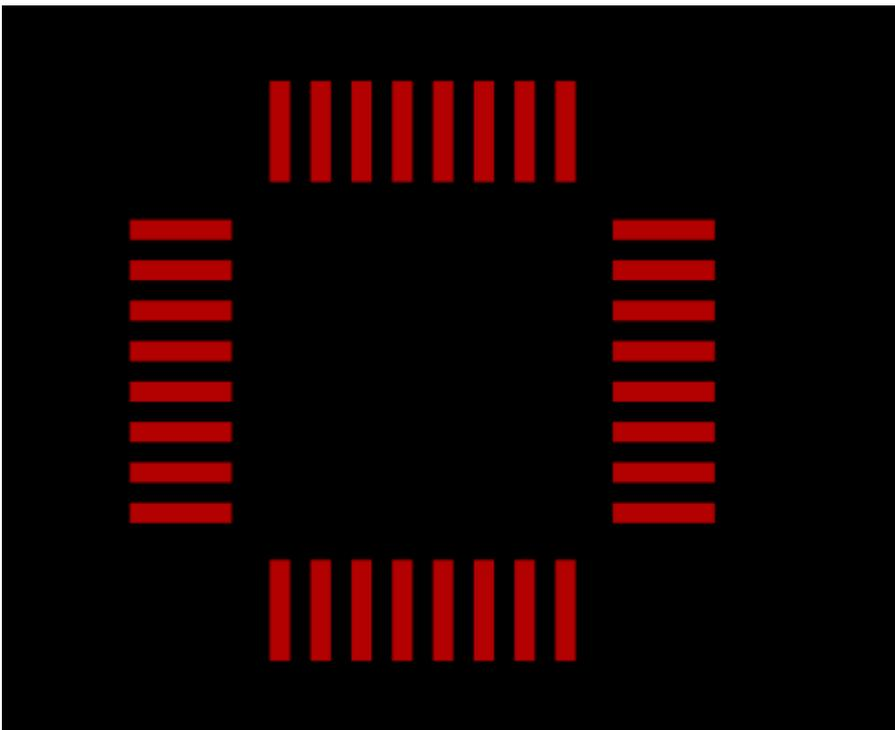
**Rectangle**—this shape is defined by width, height, and shift in X and Y relative to the origin.
