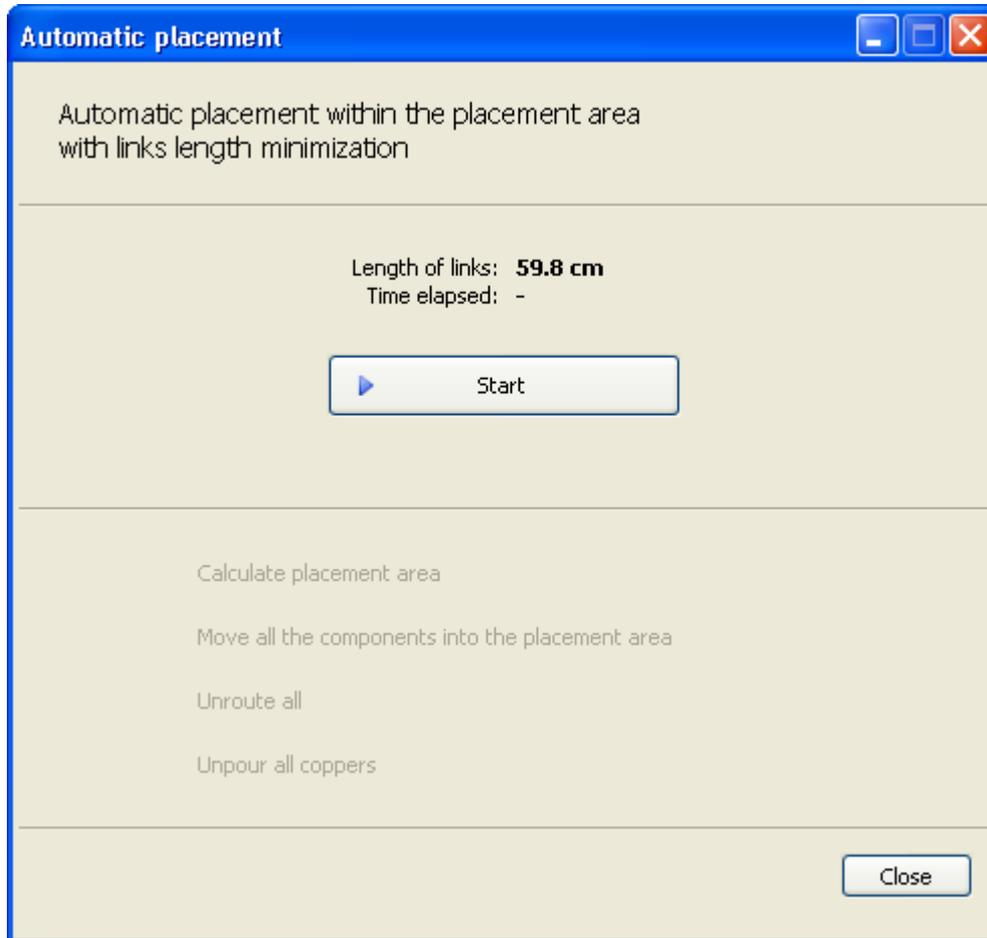
The automatic placement procedure (automatic positioning of components in the placement area while keeping the length of links to a minimum) can run only if there is at least one unfixed component; otherwise, you get a warning that the procedure cannot start (instead of a warning that the existing routes are about to be removed).
