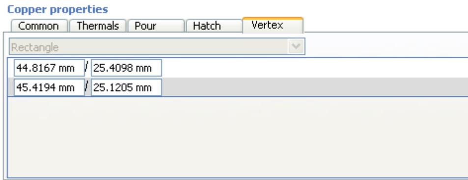
You can change the shape of a copper area in the **topology editor** or in the **Properties panel** on the **Vertex** tab by changing vertex coordinates.
