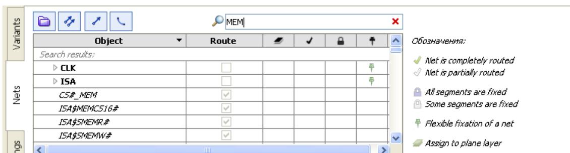
Selecting and clearing the check box in the **Route** column for a net group enables and disables routing for all nets in that group.
