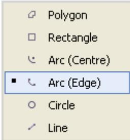
After the primitive is drawn, set the line width on the **General** tab. You can adjust the outline shape in the PCB outline editor, on the **Vertex** tab, by editing vertex coordinates.
