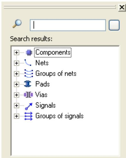
To open the Search panel, click **View ► Windows ► Search panel** or press **Ctrl+F**. This panel helps you find and select components, nets, pads and vias of specific types, and signals by name.
