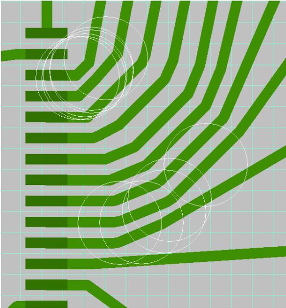
**TopoR** implements automatic calculation of the optimal wire shapes. However, due to the complexity of calculations on densely-packed boards some precision issues may occur. They are usually present around microchips with small and close-together planar pads. One tip that goes a long way in avoiding these issues is to make the nominal clearance higher than the minimal. If the problems appear anyway, there are several ways to correct them:
