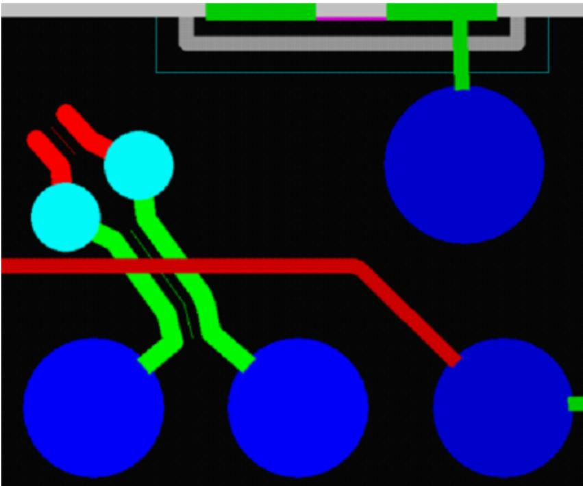
To remove overlap between the wires of a differential pair, use the net swap feature. For that, in the properties of the zipped wires, click the **Swap Nets**
