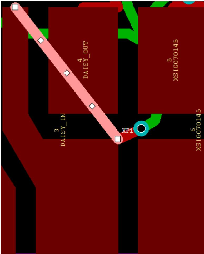
Here, the selected wire touches another pad and is not even needed at all (its only purpose is to stretch the wire to the origin); to avoid creating it, select the option above.
