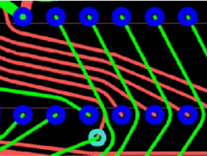
[Element moving](#) is done automatically, vias and T-points are moved to their calculated optimal positions. If a component is not supposed to be moved automatically, you should [fix](#) it first.
