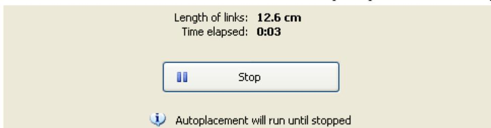
If you stop the procedure, the dialog box remains open in a paused state. Later you can either continue automatic placement where you left off or perform some auxiliary operations (calculate the placement area, move all components into the placement area, and so on) first.
