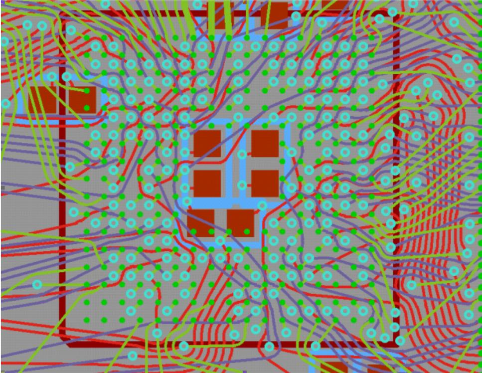
BGA components are processed in autorouting mode. When routing BGA components, the smallest interlayer via type is selected automatically. This via must be assigned to a routing rule. Two routing rules are also selected automatically: one rule for wires on the outer layer where the pads are located, and the other for wires on other layers.
