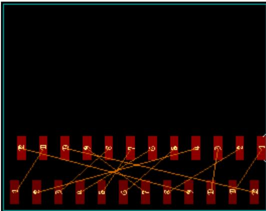
Pin positions after automatic placement (length of links reduced to 127.705 mm).
