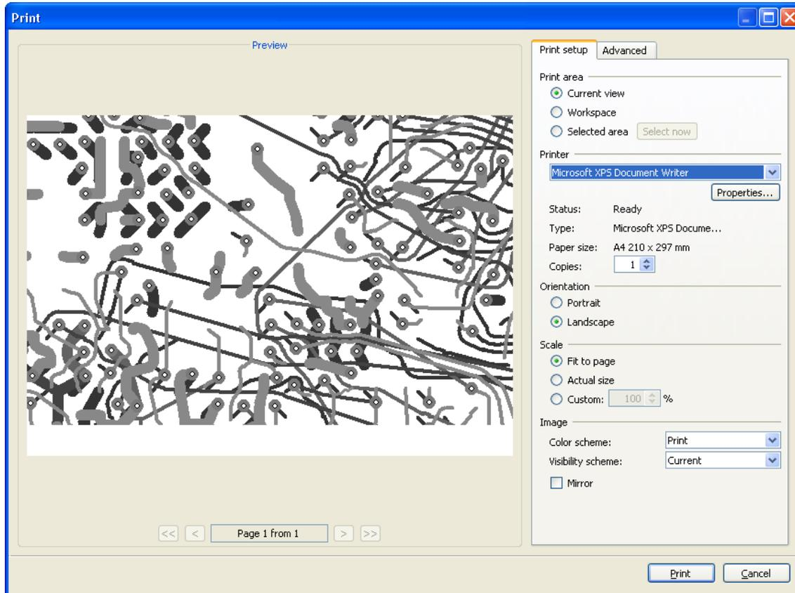
Everything that is shown on the screen goes to print. To enable or disable the display of objects, use the display control panel ([link](#)). Therefore, you can achieve the same effect without using advanced print settings. The advanced settings are provided so that you do not have to enable or disable specific objects (such as unrouted connections) every time you print.
