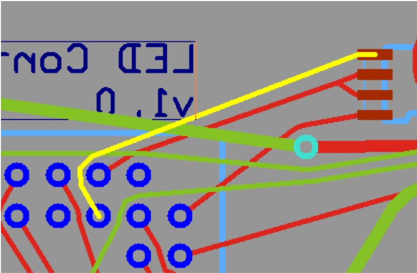
The message bar contains warnings about non-fixed elements that are over the edge of the board. At the same time, clearance violations are highlighted. The listed elements should be either fixed or moved to eliminate violations. This makes the warnings and highlighting disappear.
