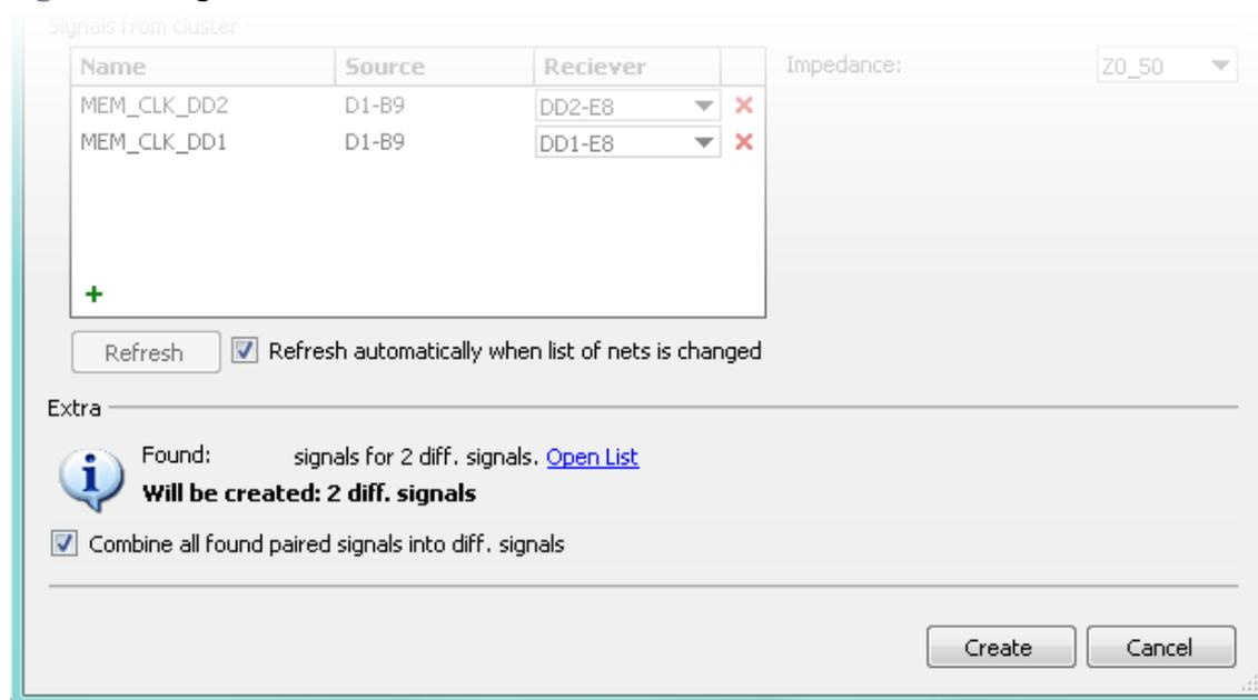
To combine the paired signals that have been found, use the **Open list** action item; in the dialog box that opens, select the differential signals you want to create. To create all available differential signals, select the **Combine all found paired signals into diff. signals** option, which is located at the bottom of the **Create signals** dialog box.
