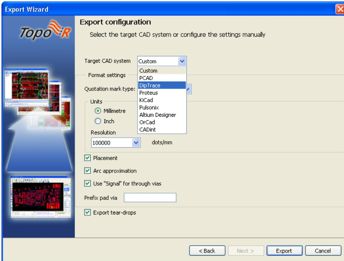
The resulting file can be imported into DipTrace by clicking **File ► Import ► P-CAD ASCII** or, in the case of **.dsn**, **Autorouter SES**.
