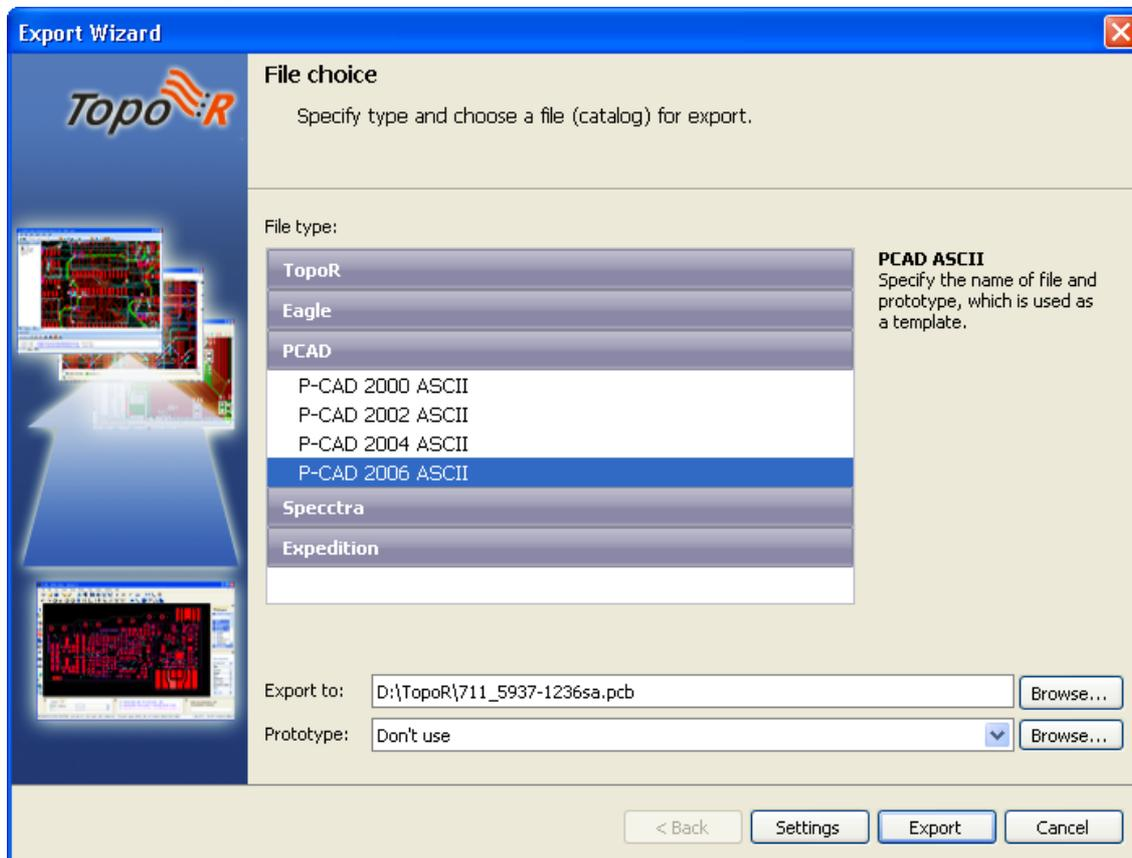
You can also use the **.dsn** or **.ses** format for the conversion, but ASCII **.pcb** is a richer format, which makes it preferable.
