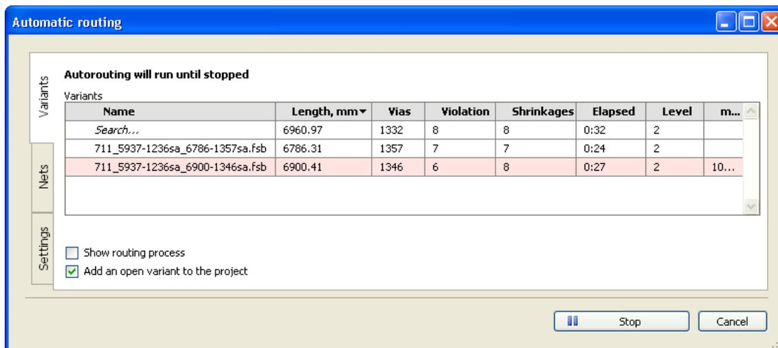
During wire rerouting, combined topology is untangled, resulting in a global minimum of vias for the current topology. You can stop optimization at any time by clicking **Stop** and continue by clicking **Resume**. To proceed with the design, click the **Open for editing** button.
