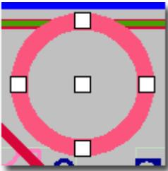
To move a circle, drag the center marker or the primitive outline. To resize a circle, drag any of the markers on the circumference. All of the above also applies to filled circles.
