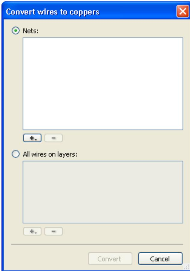
In the **Convert wires to copper Areas** dialog box that opens, select the nets where to convert wires. If you select the **All wires on layer** option, you can select one or more layers and convert all of the contained wires at once. The wire-to-polygon conversion starts when you click the **Convert** button. The completed conversion can be rolled back using the standard undo mechanism (**Ctrl+Z**).
