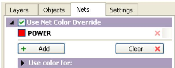
4. An option to selectively display net lines has been added (**Nets** tab in the display control panel).
