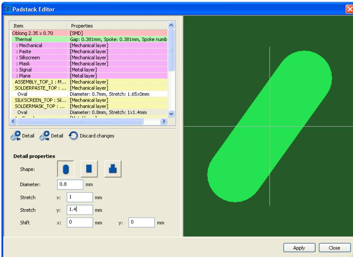
Sometimes you cannot choose the correct orientation for a pad due to conflicting use of this pad by one or more components (with different orientations).
