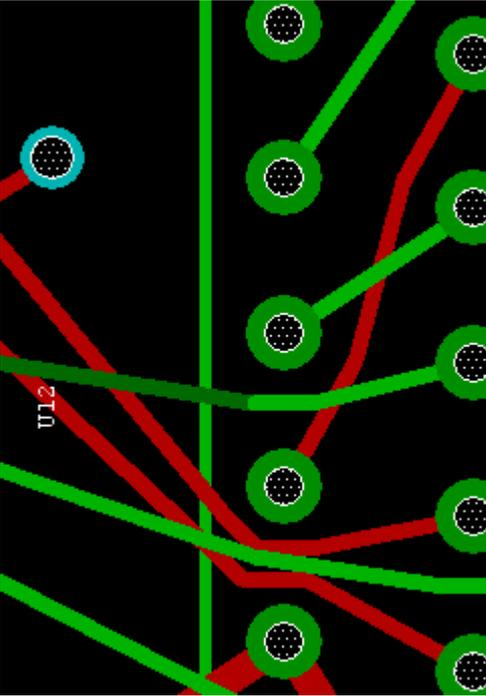
Fixed vias are also drawn in a different color, which is set in the **Objects** section in the **Display Control** panel.
